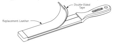
Replacement  $1^3/4" \times 9"$  leather pads can be made using a piece of leather 1/8" thick or less (7 oz or less) to ensure the stropping surface is recessed. A recessed surface will reduce the accumulation of debris when set down.
